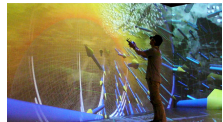
Fig. 2: A snapshot of VR visualization, or a Universe, loaded in Multiverse framework. An MHD dynamo simulation data is analyzed in this Universe by arrow vectors, tracer particles, volume rendering, etc.
