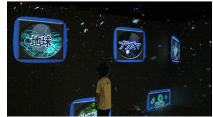
Fig. 1: A snapshot of Multiverse framework in \pi -CAVE VR system. Virtual touch screens, or virtual "Desktop" is shown. Expository movies are played in 3D space.
